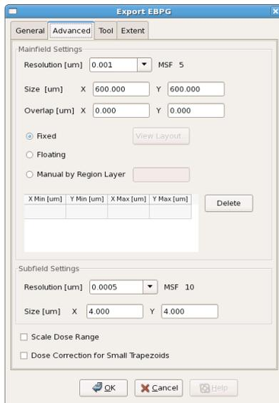
On the Advanced tab, the term "Mainfield Size" really means "block"; that is, the portion of your pattern that will be written before moving the stage to write the next portion. Your pattern will be sliced into chunks of this size. The maximum field size is always  $2^{20} \times 1 \text{ nm} = 1048 \mu\text{m}$ . This "mainfield size" on the Advanced tab is a rectangular chunk or "block" of that field.
